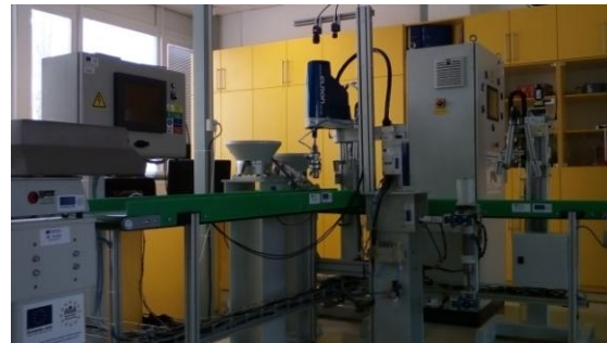
Fig.7 Assembly cell with SCARA robot and 3D object detection
