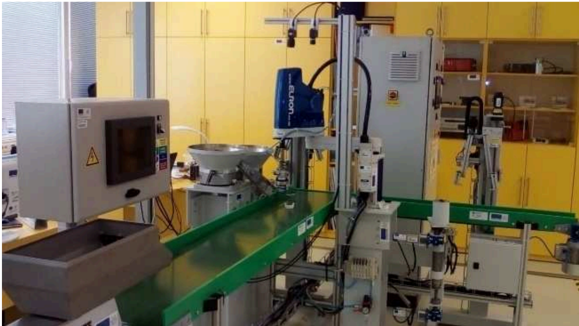
Fig. 4 Assembly cell with SCARA robot and 3D object detection
